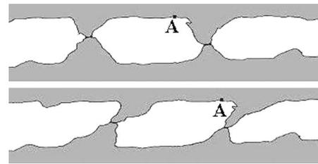
Fig. 9. A description of the adhesive junction model of Bowden and Tabor (Ref. 6). The slope of the asperities is magnified; in reality they are much smoother. Similar figures can be found in Ref. 20.
