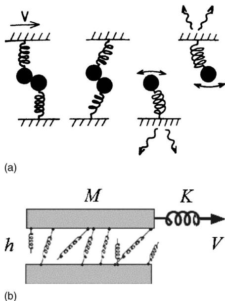
Fig. 10. Spring models for friction interactions. (a) The picture represents two asperities or atomic groups of two surfaces in contact (Persson, Ref. 6, p. 291). As the surfaces slide relative to each other, atomic groups interlock, then deform elastically, and finally slip. The rapid local motion is damped by the emission of sound waves. (b) Bond formation and rupture modeled by elastic springs with damping (Filippov *et al.*, Ref. 19).
