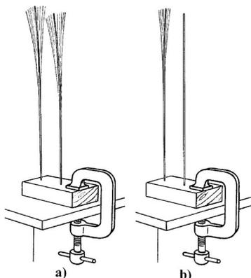
Fig. 2. Example of internal friction. (a) Two steel wires of the same size begin oscillating at the same time. (b) A little later, one wire has stopped vibrating, and the other is still oscillating. The former wire had been heated with a flame to about 800 °C and then slowly cooled, dramatically increasing its damping.
