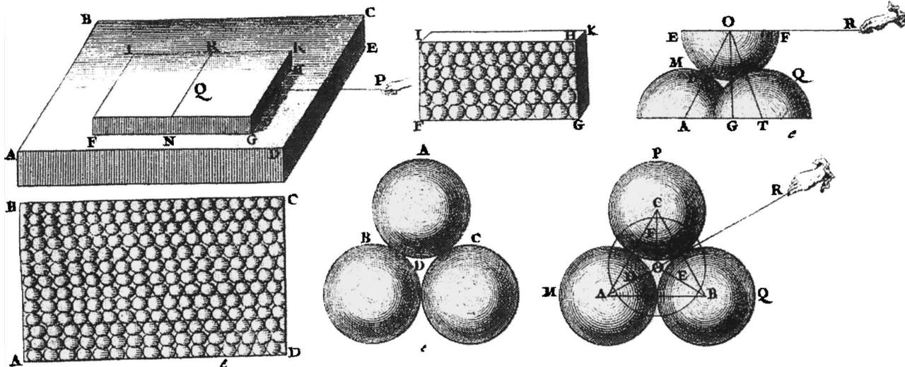
Fig. 8. In BÉLIDOR's model rough surfaces are represented by rigid spherical asperities, which interlock when two surfaces come in contact (Ref. 15). The friction force equals the force needed to move the spheres up and over each other.
