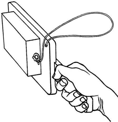
Fig. 5. A wooden paddle, which is accelerating horizontally, presses against a wooden block, thus provoking a vertical friction force, which can counteract the weight of the block.
