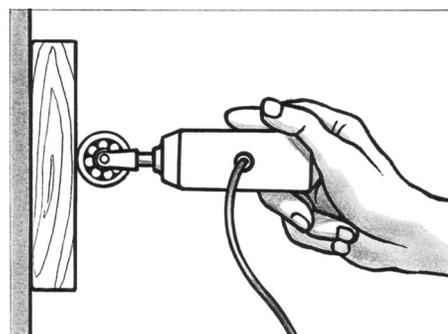
Fig. 3. A small wooden board is pressed against a wall by a force sensor. By pressing more or less, we can either prevent or allow the board to slide along the wall. The force sensor is equipped with a small ball bearing on its tip to minimize friction between the force sensor and the board.
