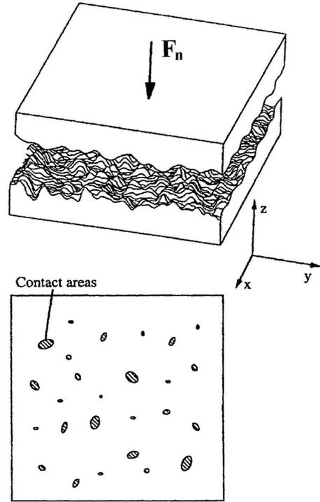
Fig. 6. The image from Bhushan, Ref. 6, p. 147, shows that the real area of contact is a small fraction of the apparent (macroscopic) area of contact.
