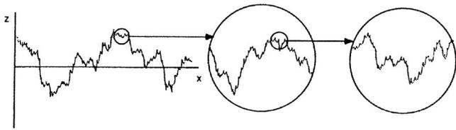
Fig. 7. The multiscale level of asperities, showing a rough fractal structure; the figure from Bhushan, Ref. 6, p. 49, represents a surface profile viewed at different magnifications. Note that the slope of the asperities is exaggerated and increases with magnification.
